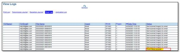
In the example above, the logs show the instance when the power failure occurred and the job recovery thereafter, as shown by log records of split e-Mails successfully sent.
