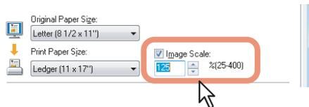
The scale can be set from 25% to 400% in units of 1%.
